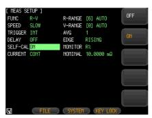
3. Use option key on the right of the LCD screen to select an available parameter.
