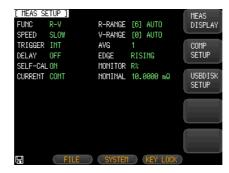
2. Press the **MEAS DISPLAY** option key on the right of the LCD screen. The MEAS DISPLAY page will display on the screen.
