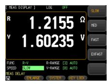
3. Use option key on the right of the LCD screen to select a parameter for this measurement item.
