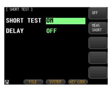
4. Press the **MEAS SHORT** and then **OK** option key on the right of the LCD screen to perform short test. User can see the short measure is in progress. And finally a message "correction finished" displays on the lower part of the LCD screen.
