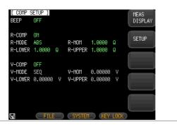
Set up buzzer 3. Use arrow keys to select **BEEP** on the [COMP SETUP] page.
