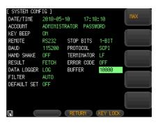
4. Enter a number from key pad, then press Enter key or press MAX option key on the right of the LCD to set up the number of data for logging.
