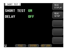
3. Use up and down arrow keys to select **SHORT TEST** on the [SHORT TEST] page.
