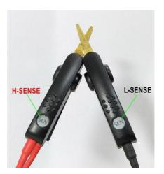
2. The SENSE terminals are clipped on the same side to complete connection of 3 points.
