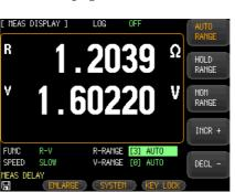
3. Use option key on the right of the LCD screen to select a parameter for this measurement item.
