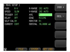
3. Use option key on the right of the LCD screen to increase or decrease average measurement frequency.
