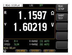
2. Press ENLARGE key below the LCD screen to enlarge resistance and voltage values on the screen.
