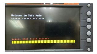
Restart the oscilloscope manually.
